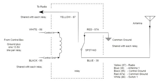
By connecting the YELLOW (87) wires together at the TRANSCEIVER SO-239 connector, I could have as many relays as necessary (in my case 5).
