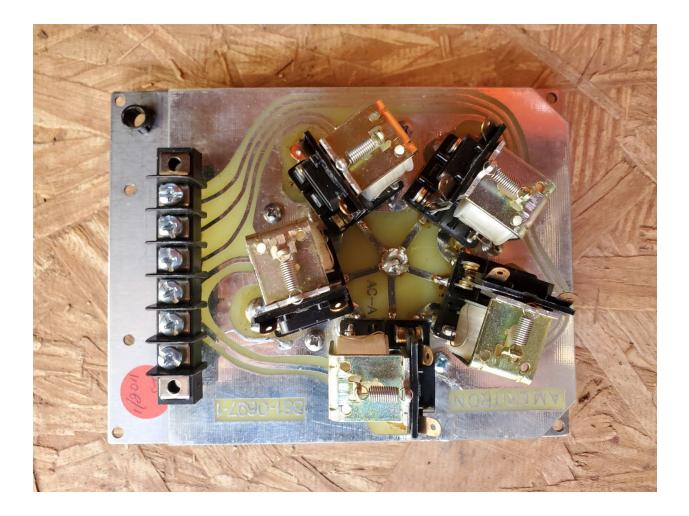
So, I need 6 SO-239 solderable connectors, a 6-terminal strip, a metal backing plate, and the relays. Note that because the relays come with pre-wired sockets, and the leads on the wires are about 7 inches, I did not need to buy any wire. Also, in my case the existing box was too small to allow me to use the sockets that came with the relays so I opted to solder slip on connectors to the wires and not use the supplied sockets. All this would be even easier in a larger box using the sockets!
