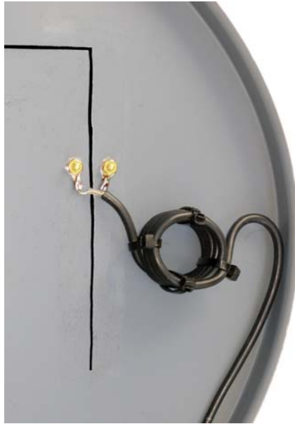
Figure 6: Coax attachment, 4½ in. from end. Note six turn coiled-coax 1:1 choke balun.
